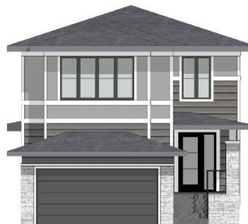
8' garage door – secondary material applied
