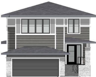
7' garage door – elevation looks disproportionate
